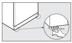
■ To align the appliance, adjust the front feet using the spanner supplied.
